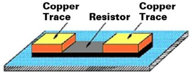
Figure 3: Thin film embedded resistor.
