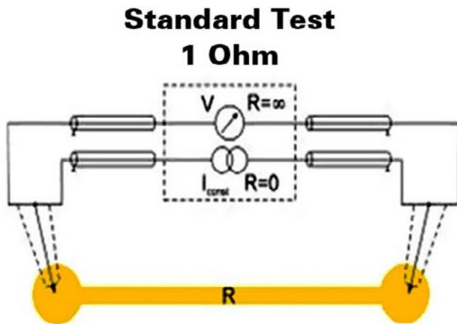
Figure 5: Resistor measurement with current limiting.
