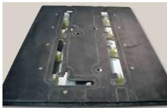
Figure 2: Fixture with dams.
