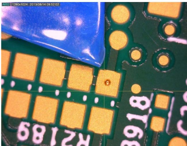
Figure 1: Pin damage.
