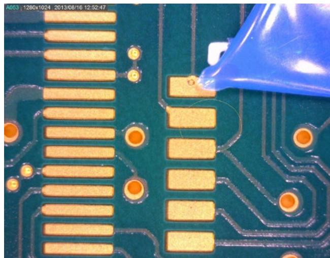
Figure 2: Pin damage.
