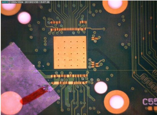
Figure 5: Wire-bond damage.
